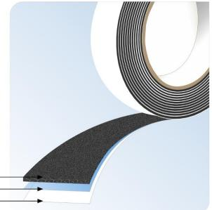
Carrier, closed-cell foam rubber (CR), black -Adhesive, acrylic dispersion -Liner, siliconised paper, white -
