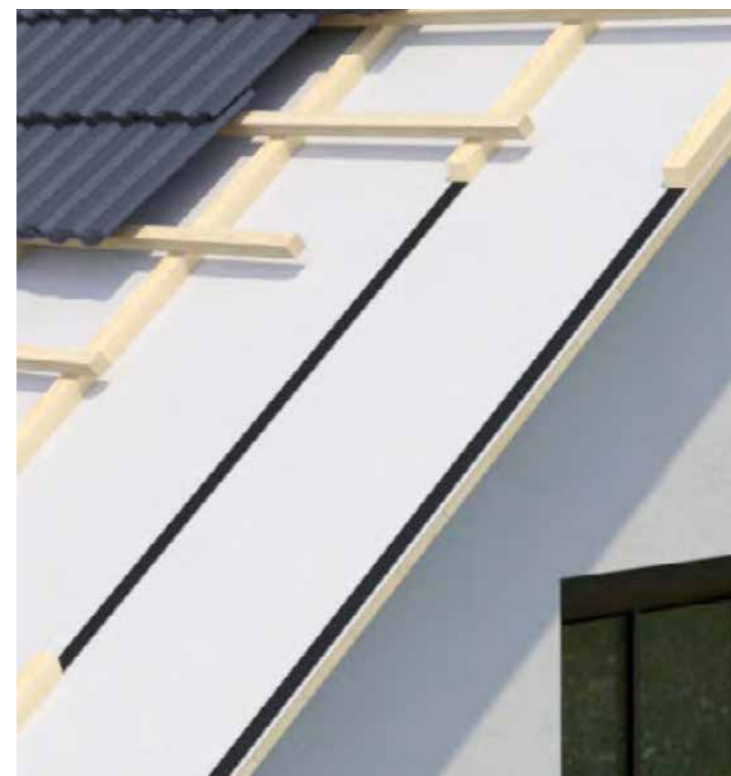
Application as nail sealing tape
