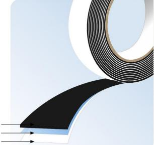
carrier, PE-foam, 0,4 mm, black \_\_\_\_\_ adhesive, UV-acrylate \_\_\_\_\_ liner, siliconised paper, white \_\_\_
